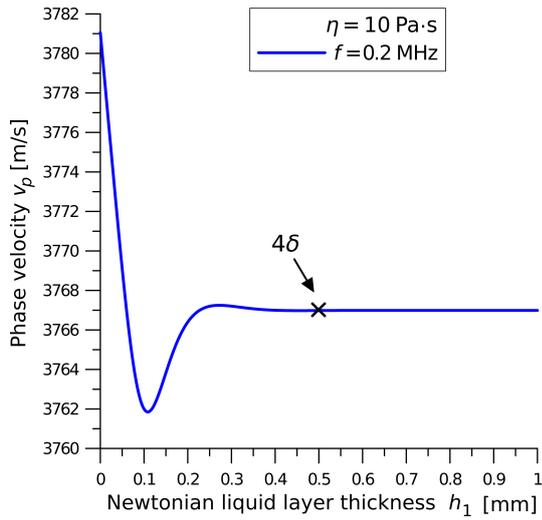
Fig. 4. Phase velocity  $v_p$  of the Love wave versus finite thickness ( $h_1$ ) of the Newtonian liquid layer, that loads the waveguide surface.  $f = 0.2$  MHz.  $\delta$  is the penetration depth of the bulk SH wave into a Newtonian liquid.
