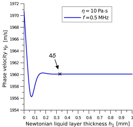
Fig. 5. Phase velocity  $v_p$  of the Love wave versus finite thickness ( $h_1$ ) of the Newtonian liquid layer, that loads the waveguide surface.  $f = 0.5$  MHz.  $\delta$  is the penetration depth of the bulk SH wave into a Newtonian liquid.
