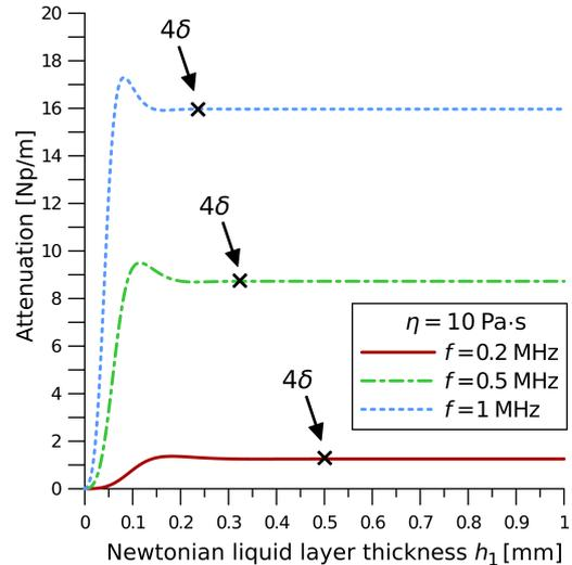
Fig. 7. Attenuation  $\alpha$  of the Love wave as a function of Newtonian liquid layer thickness  $h_1$ .  $f = 0.2, 0.5$  and  $1$  MHz.  $\delta$  is the penetration depth of the bulk SH wave into a Newtonian liquid.
