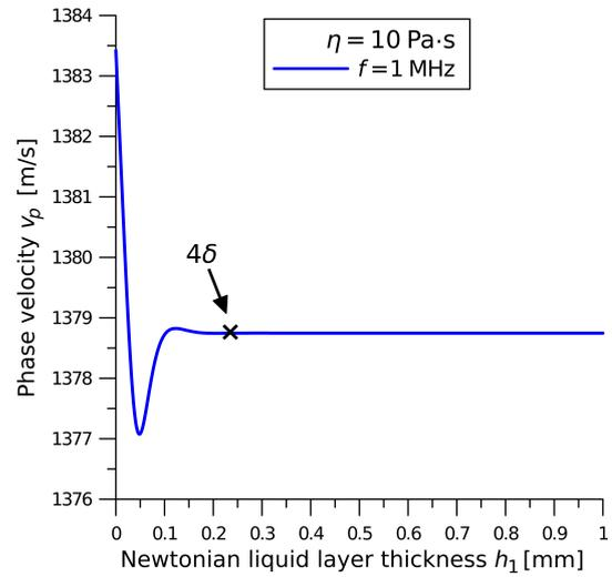
Fig. 6. Phase velocity  $v_p$  of the Love wave versus finite thickness ( $h_1$ ) of the Newtonian liquid layer, that loads the waveguide surface.  $f = 1$  MHz.  $\delta$  is the penetration depth of the bulk SH wave into a Newtonian liquid.
