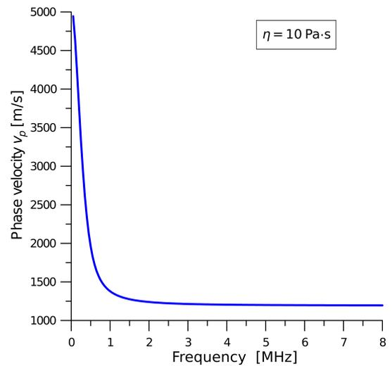
Fig. 2. Dispersion curve of the phase velocity of the Love wave propagating in the layered waveguide of Fig.1. Thickness of surface gold layer  $h_2 = 0.1$  mm. Newtonian liquid of viscosity  $\eta = 10$  Pa·s that loads the upper surface of the gold surface layer is a semi-infinite half space.
