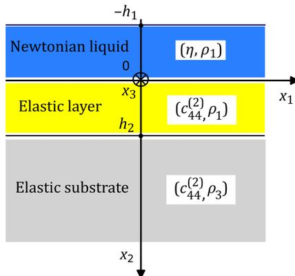
Fig. 1. Cross-section of the analyzed lossless Love wave waveguide loaded with a lossy Newtonian liquid. Love surface waves propagate along the  $x_1$  axis. Shear horizontal (SH) mechanical displacement  $u_3$  of the Love wave is directed along the  $x_3$  axis.
